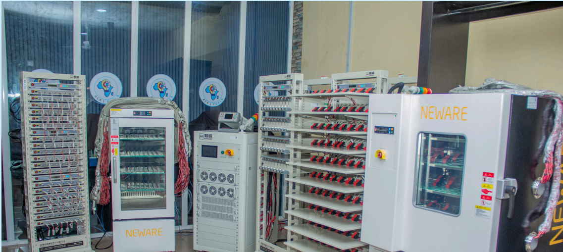
The battery testing system and aging/constant temperature chambers enabling precision testing, controlled performance evaluation, and advanced battery research at ACE-FUELS ElectroLab X
